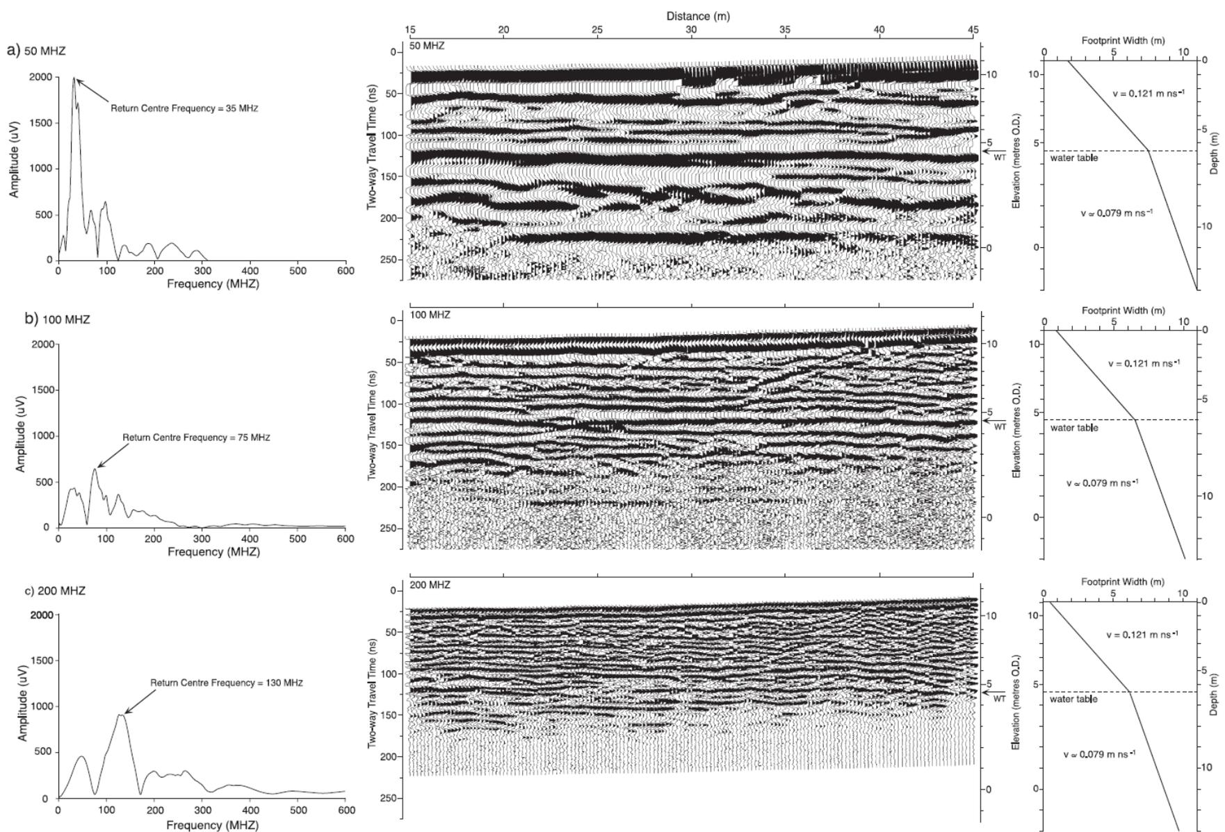
Fig. 7. Return-frequency spectrums, radar reflection profiles and radar-footprint size variations with depth for data collected along the same shore-parallel transect across sand-and-gravel-rich beach ridge-plain deposits, Beckfoot, outer Solway Firth, northwest England using antennae with nominal centre frequencies of (a) 50 MHz, (b) 100 MHz and (c) 200 MHz. Note expansion of the elevation axis beneath the water table (WT) due to the decrease in radar wave velocity.
