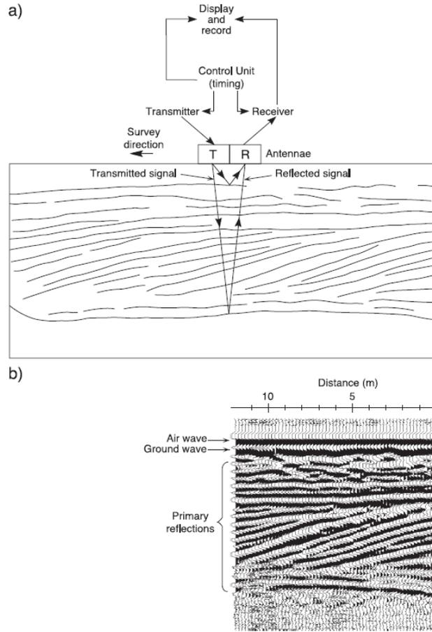
Fig. 3. GPR data acquisition and the resulting radar reflection profile. (a) Data acquisition at an individual survey point, showing GPR system components and subsurface reflector configuration. (b) Radar reflection profile resulting from sequential plotting of individual traces from adjacent survey points. Position of the airwave, ground wave and primary reflections are indicated. Modified from Neal and Roberts (2000).
