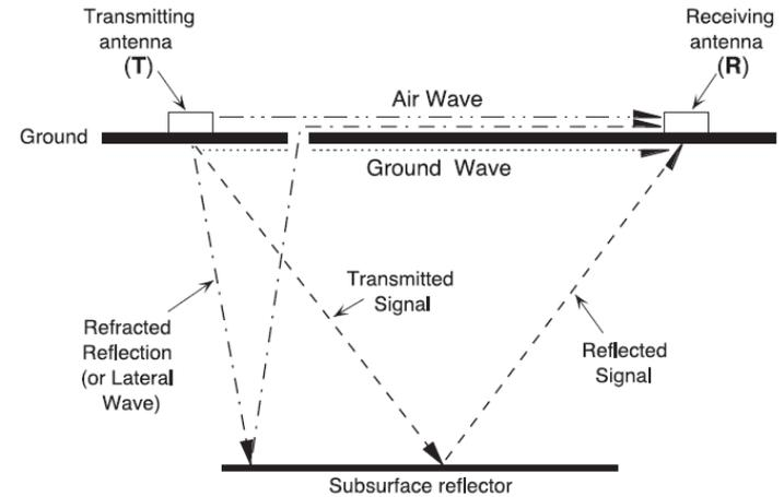
Fig. 4. Ray paths between transmitting and receiving antennae for the airwave, the ground wave, a lateral wave and a reflected wave. Modified from Fisher et al. (1996).
