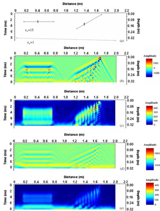
Figure 3. Synthetic data: (a) model, (b) raw data with air-filled fracture, (c) time domain processed data with air-filled fracture, (d) raw data with moist-material-filled fracture and (e) time domain processed data with moist-material-filled fracture.
